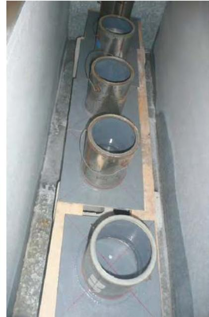
ASTM D1970 test apparatus. This test measures the ability of a barrier material to self-seal around two nails in a manner sufficient to prevent a column of water from seeping through the penetration.
