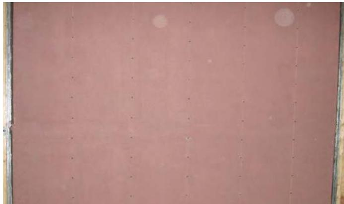
*ASTM E2357 panel made using ENERSHIELD-I with 75 penetrations*
