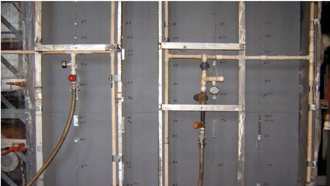
*ASTM 331 test apparatus*
